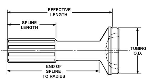
If tubing insert diameter requires machining to fit a tube, machine it to a diameter of .007" to .010" larger than the inside diameter of the tube for proper press fit.
