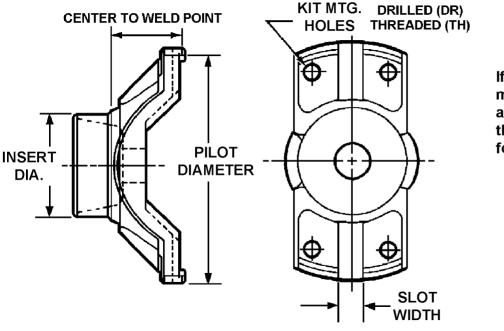
If tubing insert diameter requires machining to fit a tube, machine it to a diameter of .007" to .010" larger than the inside diameter of the tube for proper press fit.
