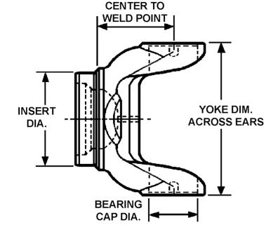
If tubing insert diameter requires machining to fit a tube, machine it to a diameter of .007" to .010" larger than the inside diameter of the tube for proper press fit.
