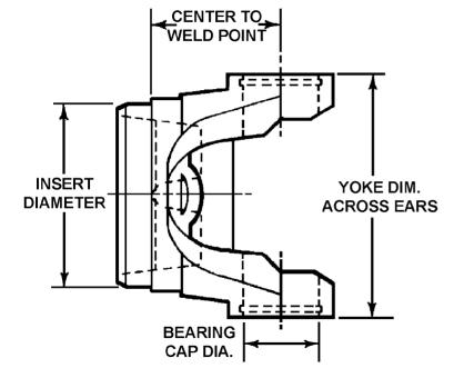
If tubing insert diameter requires machining to fit a tube, machine it to a diameter of .007" to .010" larger than the inside diameter of the tube for proper press fit.
