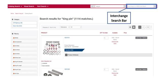
4. Find King Pin Kit by Axle Tag (Meritor axles only). Locate the silver axle tag on the steer axle. Record the axle model from the tag and enter it into the MeritorPartsXpress part number search bar. Click on the Axle Model in MeritorPartsXpress. Finally, click on the "Service Kits" tab if available to see any related service kits.
