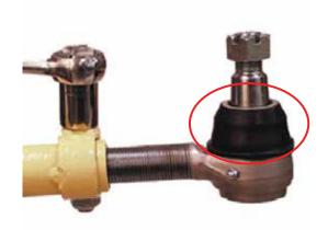
• Check that tie rod end is threaded correctly into the cross tube and installed deeper than the end of the cross tube slot.
