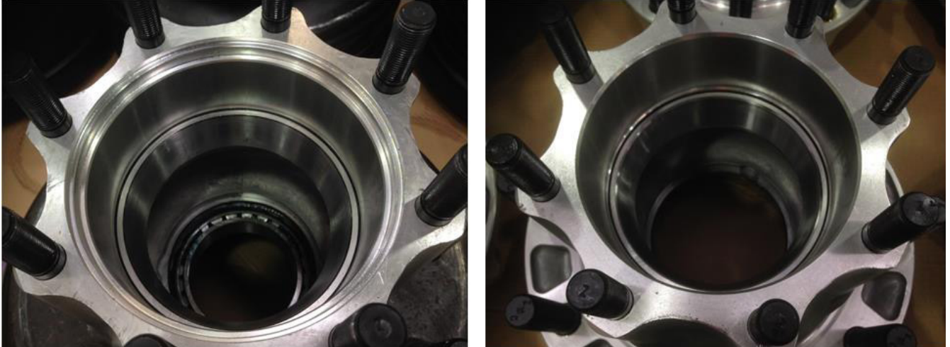
Figure 3 – Comparison of current (left hand) and new (right hand) machining
